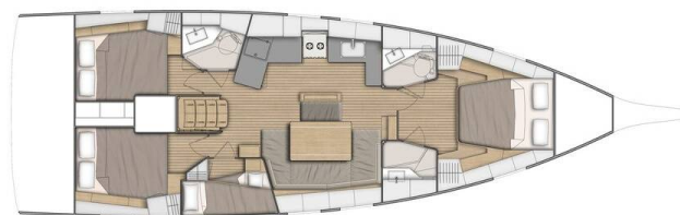
OCEANIS 46.1 - layout 4 CABINS & 2 HEADS
